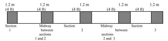
Test load: The maximum test load applied to the prescribed test pattern shall not exceed the concentrated load capacity (or for scales manufactured prior to January 1, 1989, the rated section capacity).
