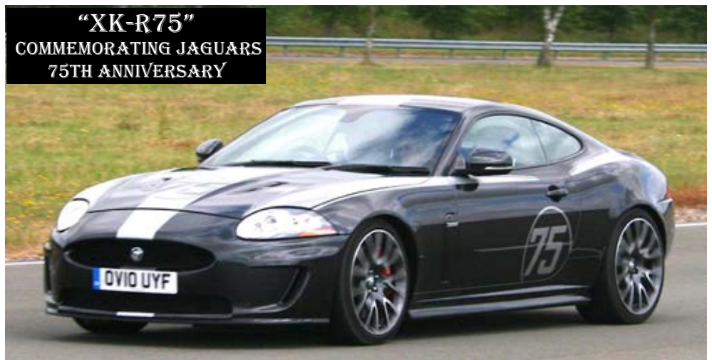
The 2010 "XK-R75 Goodwood LE" version was built to commemorate Jaguar's 75th anniversary. The cars were tuned and calibrated in partnership with the RSR ("Rocketsports Racing") engineering team that developed the all conquering American Trans-Am XK. The 75 cars were finished in Stratus Grey exterior paint with an optional graphics pack.
