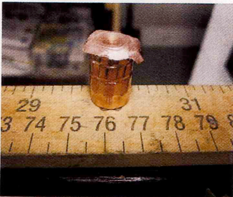
A recovered .500-calibre 470-grain copper hollow-point projectile, which penetrated 30" through the bullet box test media.
