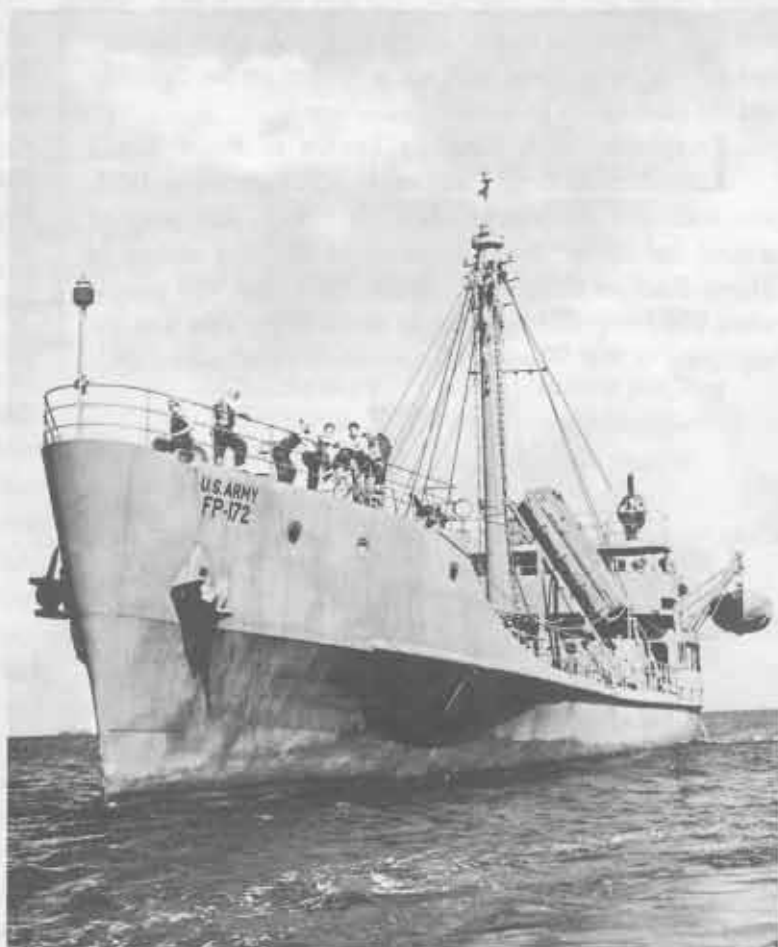
An Army FS (freight supply), formerly FP (freight personnel) ship similar to the one George Alton was stationed on following his duty aboard the PC 469 . Thousands of Coast Guardsmen made up the crews of hundreds of these hard-working 180-footers. Known as "island hoppers," because of their shallow draft, these vessels could penetrate into the devious maze of islands, atolls and hidden reefs to deliver troops and supplies to far Pacific bases
