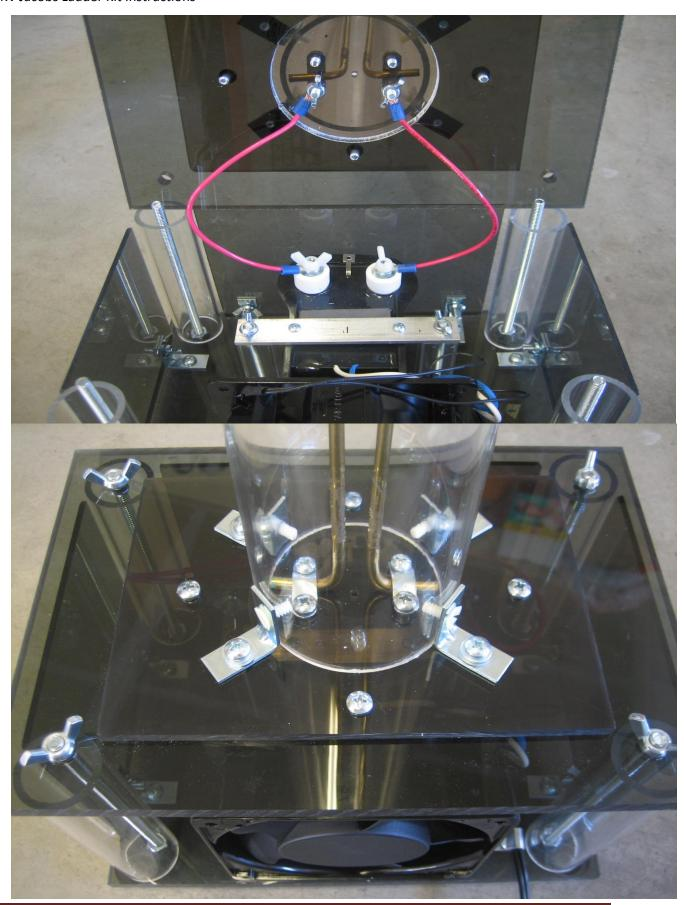
9) Screw on the top plate with the larger wing nuts and prepare for an initial test.
