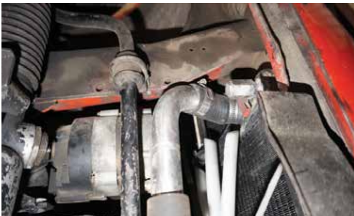
Lower hoses to radiator looking up from under the car
