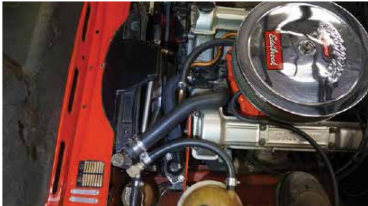
Lower hoses to radiator looking up from under the car
