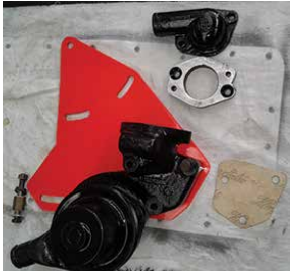
Saloon water pump, mounting stud & pieces on red mounting plate →
