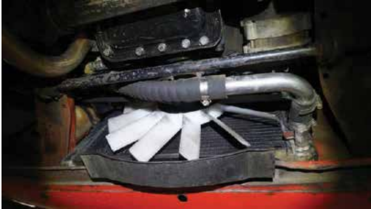
Hose and pipe underneath the car and looking down on the engine. You can see the revised heater pipe ( rubber and copper "S" bend).
