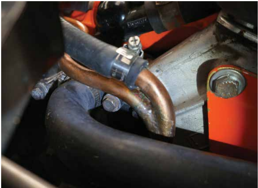
Close ups of bypass hose and copper pipe combination for heater operation. Below also shows LHT and corner of mounting plate.
