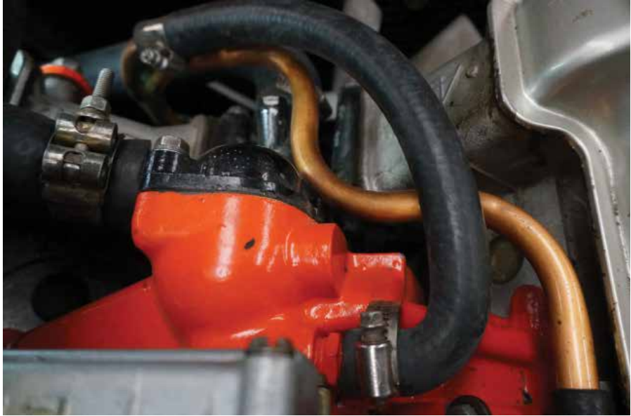
Close ups of bypass hose and copper pipe combination for heater operation. Below also shows LHT and corner of mounting plate.
