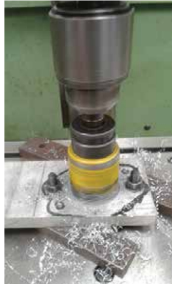
← Milling the slots in the mounting plate
