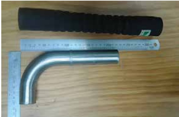
← Shows dimensions of convoluted hose & stainless steel water pipe
