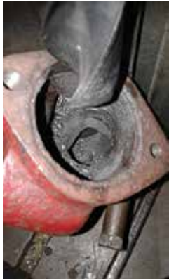
← Drilling out the saloon pump to increase water flow
