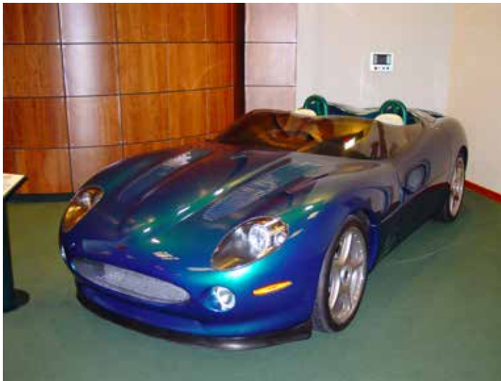
One car which attracted a lot of interest was the XK 180 Concept car. Built in 1999 to celebrate the 50th anniversary of the XK 120. The 4.0 litre supercharged V8 had a claimed top speed of 180 mph. Only two XK 180 roadsters were built, one LHD and the other RHD.
