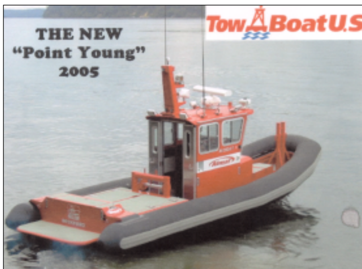
CAPT Charles Meyer, owner of Lake Tow, a marine assistance company on the Lake of the Ozarks, named his new 27-foot rescue towboat Point Young. Meyer served aboard the USCGC Point Young in 1969, until her turnover to the Vietnamese Navy in March 1970. The new Point Young is a rigid-hull inflatable with a deep "V" hull.
