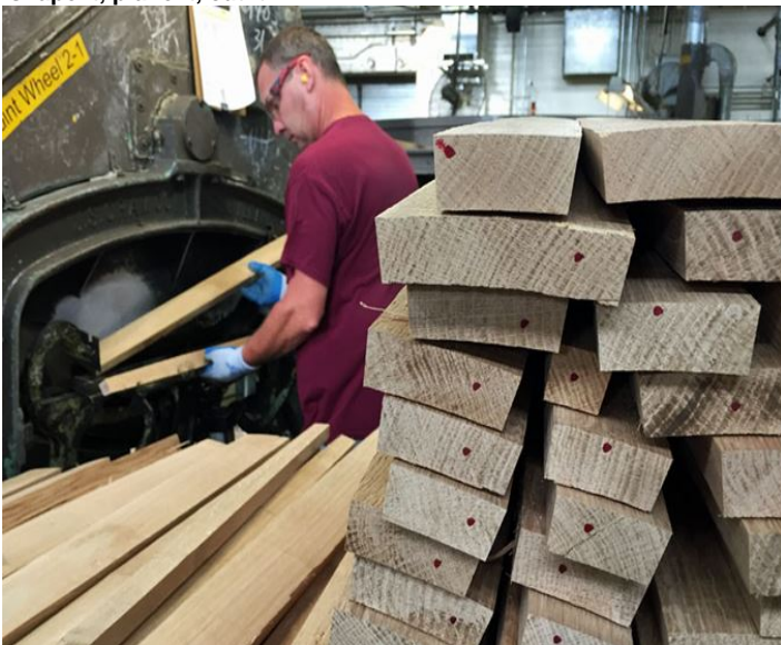
Perfect fit: The stave edges are shaped so they can slot neatly together into a barrel shape
