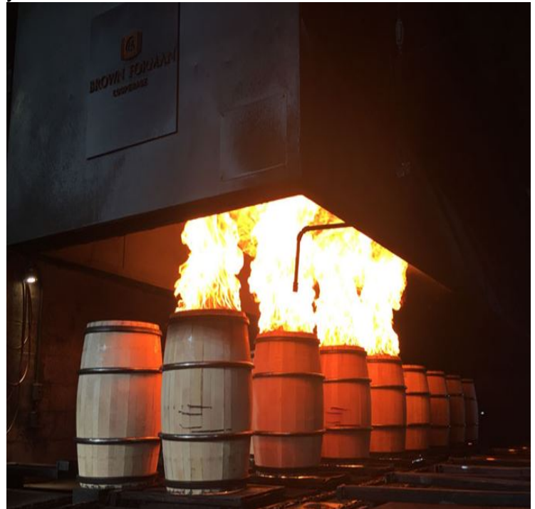
Fierce flame: The barrels are set alight to produce a layer of char on their interior surface
