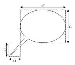
The distance between these two parts that you have to enter in the object properties is represented in the upper drawing as x1 and y1.
