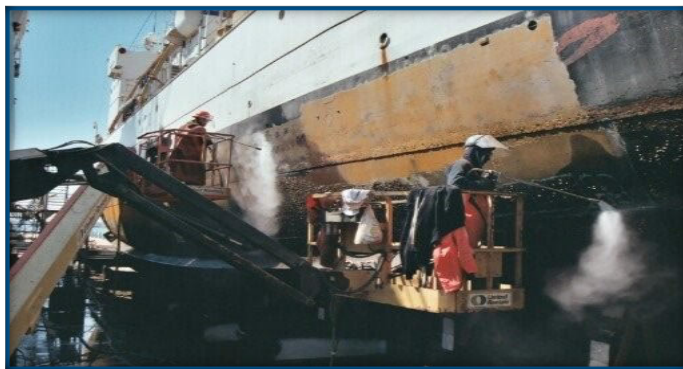
Sandblasting the hull USCGC TANEY
