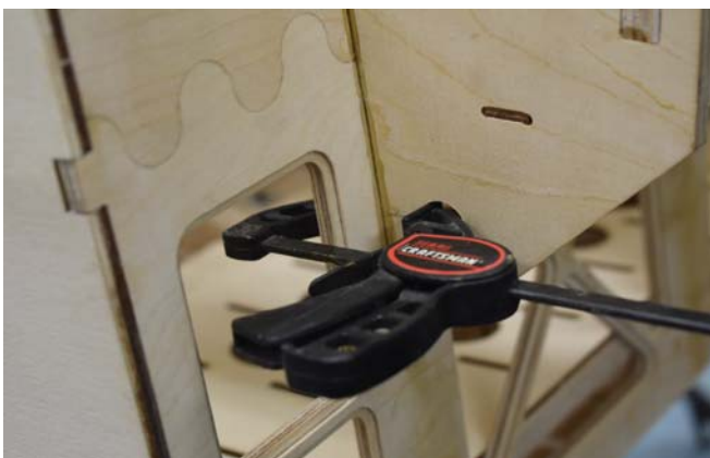
192. Epoxy (30 min.) 3/4" balsa triangle stock around the engine box behind former F2.
