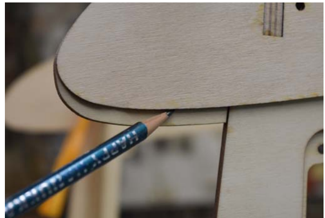
134. Mark the bottom overhang of FW1 assy. (as to not add glue to this area) and glue to the inside of FW5 .
