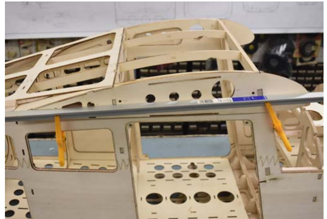
133. Clamp on a 90° angle that is straight and flat to FW5 . (These can be purchased at your big box stores. 1" to 2" L x 1/8" thick).
