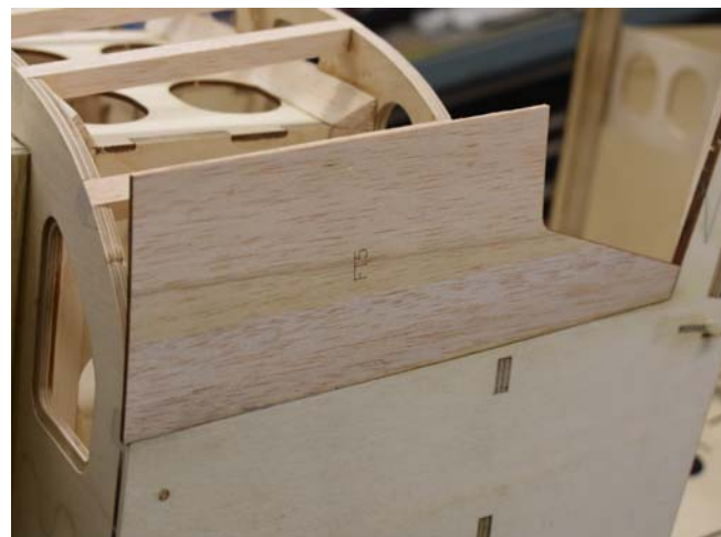
195. Glue balsa FT5 on edge to the fuselage side as shown. Allow to cure before proceeding. Repeat for the other side.
