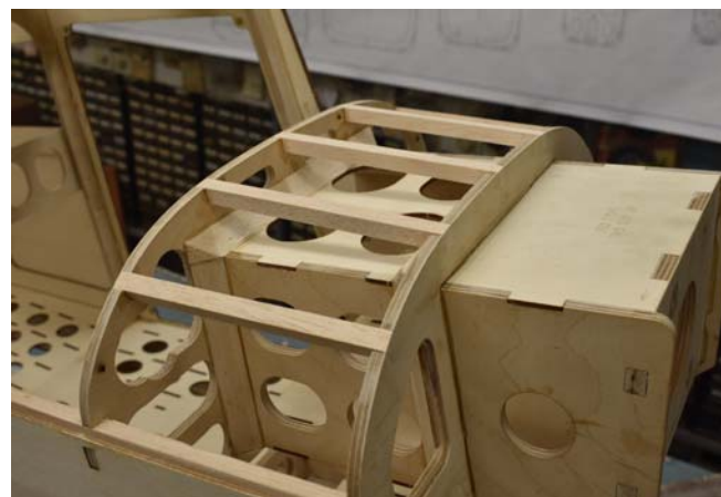
194. Glue in 3/8" square balsa sticks. Trim and sand both ends flush.
