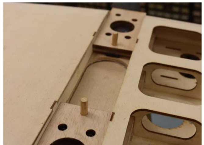
159. Place assemblies back onto the landing gear. Insert but do not glue in two 5/16" diameter dowel alignment pegs. Glue on top FL4C and remove dowels.
