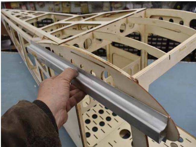
131. Sand the sides of FW5 smooth and flat from any protruding parts or glue.
