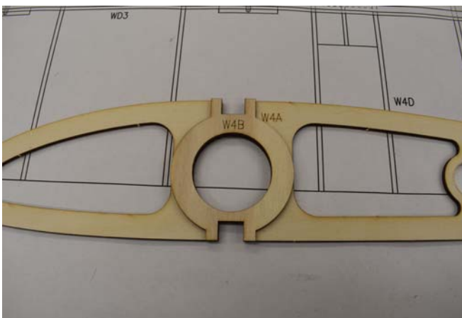
7. Glue W4B and W4C to rib W4A . (Mirror image for Left Wing)
