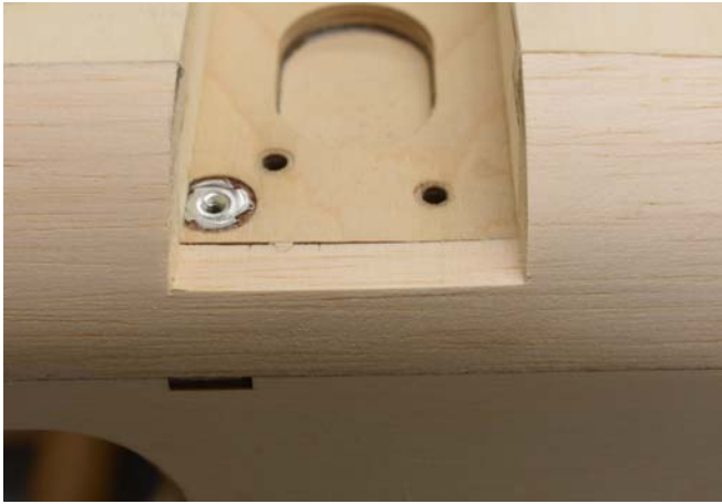
157. Bolt on the landing gear halves with 10-32 x 1" long socket head bolts and lock washers. (Pictures shows a one piece gear which is not available).
