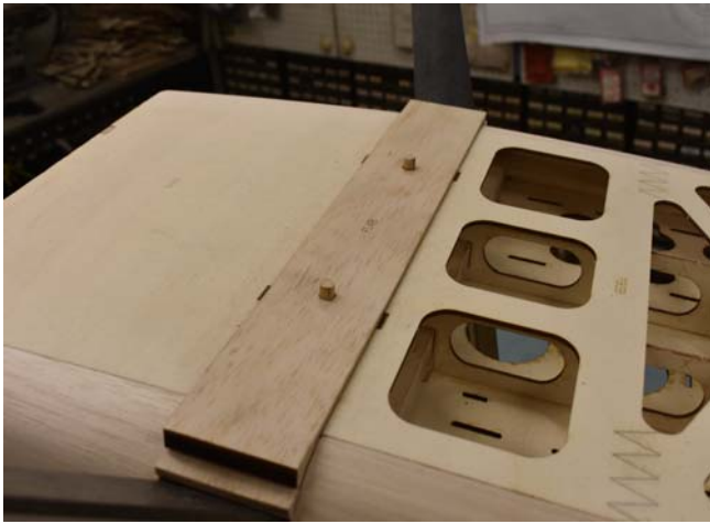
160. Drill a 5/64" diameter pilot hole into the landing gear plate and secure the cover down with two #4 x 1/2" long screws.
