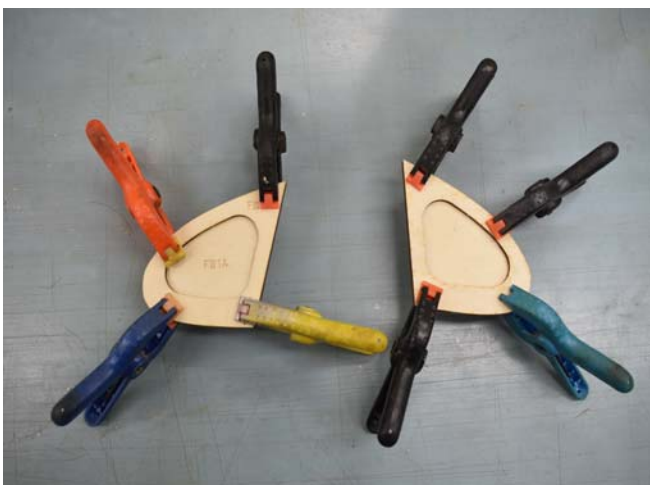
132. Glue FW1B onto FW1A . Make a left and right hand assembly.
