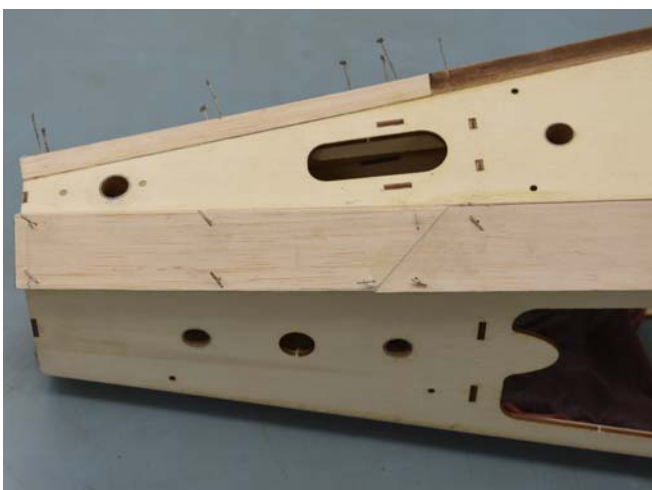
145. Glue in a long FC3 first followed by a short FC3 . Draw a straight line from the rear to the front and trim away excess.
