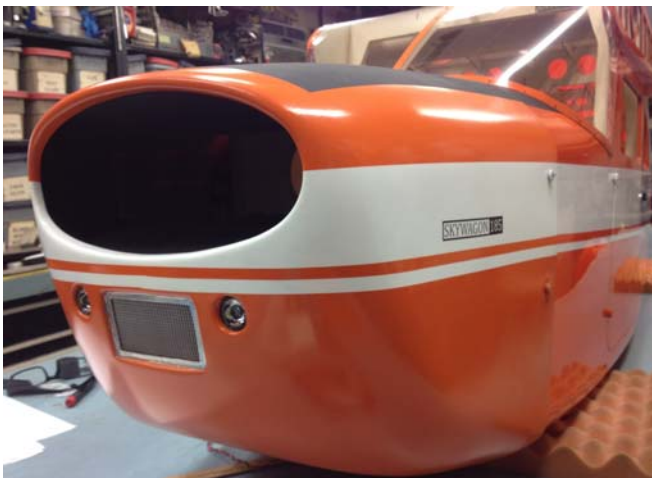
Cooling baffles painted flat black and screen added to air inlet. Screen is glued in from the inside of the cowl.
