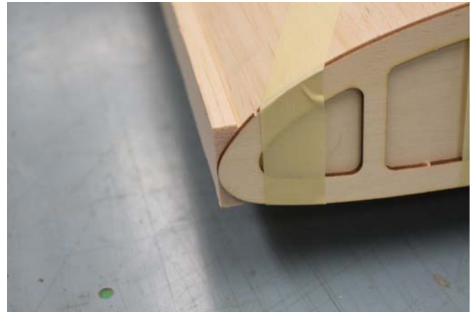
108. Temporary tape on W1A and shape the leading edge.
