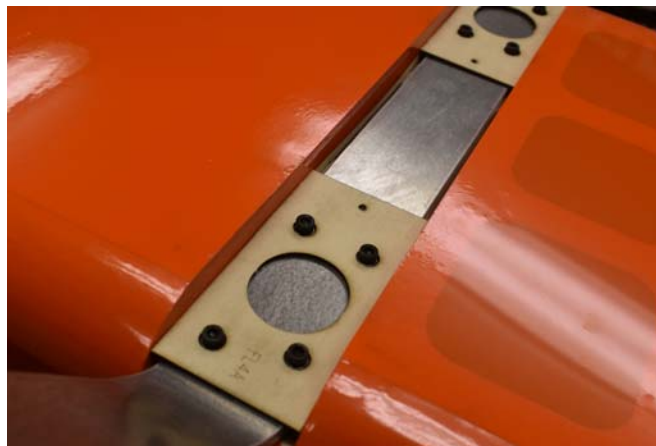
158. Lay down onto the gear FL4A (Holes lining up with the bolts) and then glue on FL4B . If necessary sand a radius to match the radius of the landing gear.
