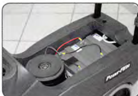
Easy access to motor and battery
