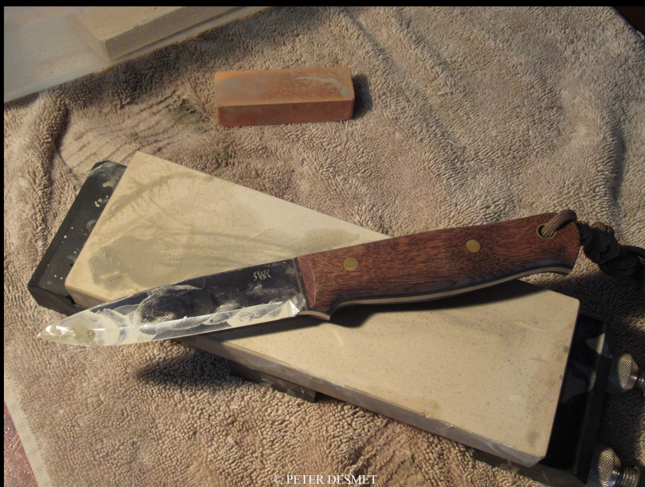
Bench sharpening set-up with Japanese water stones. ON, Canada.
