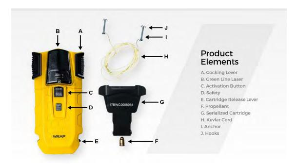
Each cartridge contains an eight-foot Kevlar® tether. Each tether has a 4-hooked anchor on either end. Quick refresh enables reload time of 3-8 seconds. Powered by a .380 partial charge blank, the BolaWrap® exits at 513 feet per second and wraps between 1-3 times around the subject at a range of 10-25 feet. Kinetic energy decays rapidly with distance after discharge.
