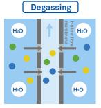
Oxygen and other gases in the water are removed through the membrane
