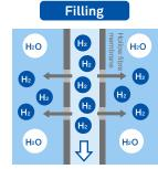
Hydrogen is passed through the membrane and dissolved in water
