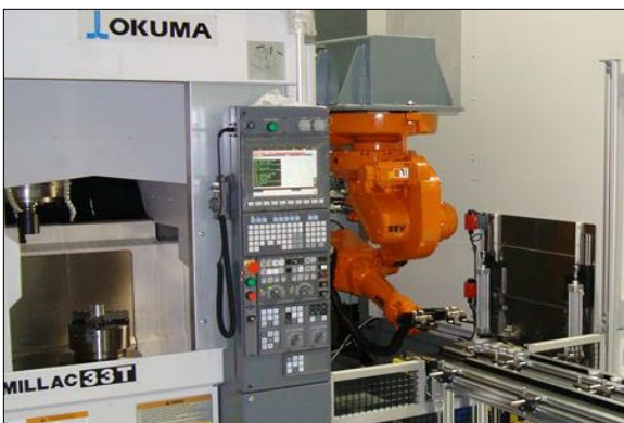
Robot Feeding Parts In & Out of CNC Machine
