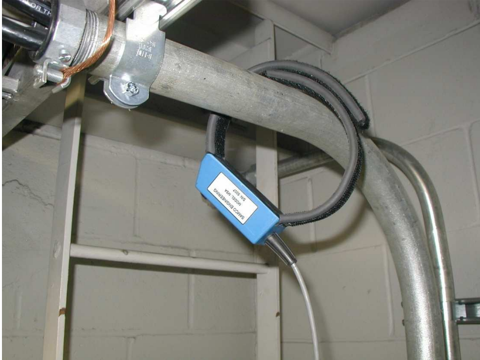
Fig. 3, Large Magnetic Sensor (MSA) around a conduit that has several conductors
