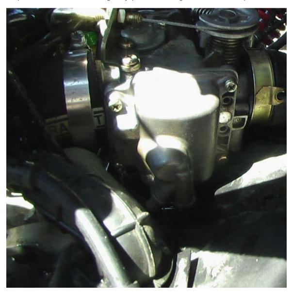
5) Remove the screws on each corner of the bottom of the bowl to remove the float cover. Gas will definately spill at this point if the bowl wasn't properly drained earlier.
