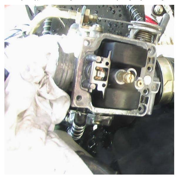
7) Using a flat head screw driver twist counter clockwise to remove the button type main jet. If the brass base try's to come off with the button jet you will need to use a small wrench (not pictured) to hold in it place while you unscrew the jet. (see detailed picture of jet in and jet removed)
