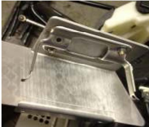
6. Unplug the fan and attach the fuse box back on the factory bracket.
