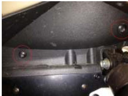
4. Remove the fuse box from the bracket that's attached to the coolant reservoir so the bracket can be unbolted from the coolant reservoir. Once the bracket is removed the reservoir can be re-attached.
