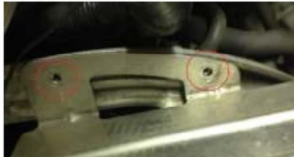
3. Remove the two bolts that secure the coolant overflow tank to the sled.
