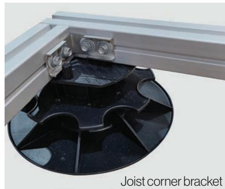
**Step 1** - Understand the spacing's required for the finished product going on top. For composite decking in residential setting using our 38mm aluminium joist, the spacing for the aluminium joist will be 400mm centres and the pedestal spacing will be 700mm.
