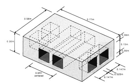
Fig. 2. Dimensions of stone crab modules used to control den quality while manipulating dispersion of den patches. Each end has 2 blind holes while holes in long sides are open-ended, for a total of 6 dens per module
