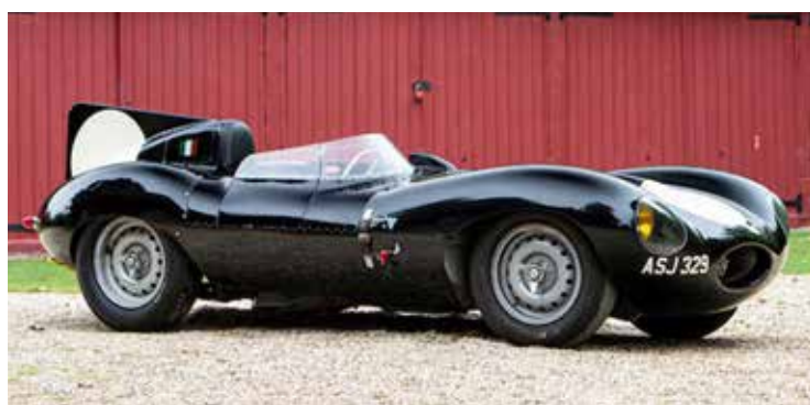
1956/1980s D-Type. 'XKD 570' was dismantled for parts by Jaguar. In 1980s this finned 'Shortnose' D-Type was assembled from assorted original and reproduction parts. Sold AU $1,510,366 (£799,000).
