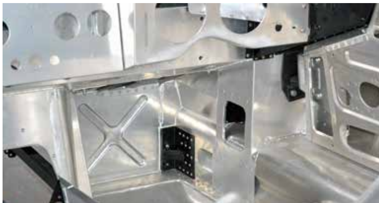
A work of art, not just a car in the making. The correct period rivets were used, and along with specific aluminium sheeting imported from the U.S. They provided a final result to please the most fastidious of inspections.
