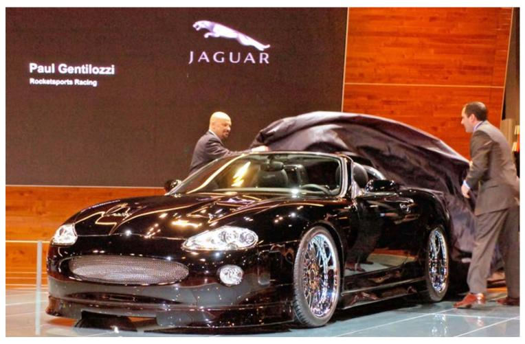
Rocketsports racing developed this modified version of the outgoing 2004 XK model. Known as an XK-RS, the car made a world debut at the Chicago Auto Exhibition. Tested in a wind tunnel this concept car features deeper front and rear spoilers, wider wheel arches and the engine enlarged to 5.0 litres. This one-off XK-RS Concept 550 horsepower convertible had a claimed top speed of 200mph.
