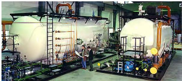
chlorides come from the reservoir water and are also dissolved in the oil. The desalters will be placed after the first or second stage separator depending on Gas Oil Ratio (GOR) and water cut. *Photo: Burgess Manning Europe PLC*
