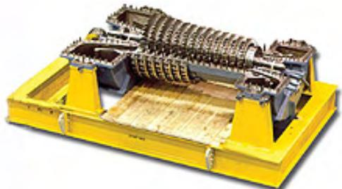
Applications include air compressors and cooling compression in LNG plants. *Axial rotor photo: Dresser Rand*
