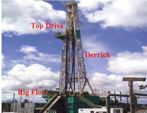
The main components of the drilling rig are the derrick, floor, drawworks, drive and mud handling. The control and power can be hydraulic or electric.
