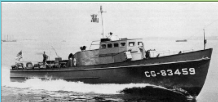
Good shot of the subject. Note the boxes on either side of the pilothouse which are storage for the 7.2 rockets. This has the plywood pilothouse.
