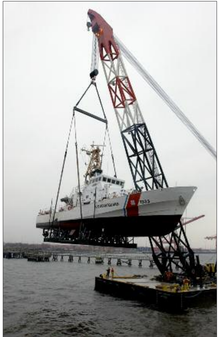
110-foot cutter ADAK being loaded on board a Military Sealift Command vessel destined for the Middle East. (Courtesy of U.S. Coast Guard)
