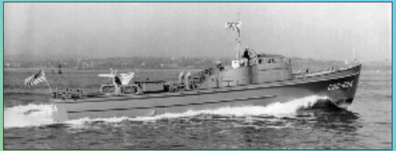
Starboard side view of an 83'er underway. Note the pilothouse. This was the bronze version, early production. Bronze started to run short during the war, so later versions were fitted with a plywood pilothouse which was more angular and less of a chamber on the roof.
