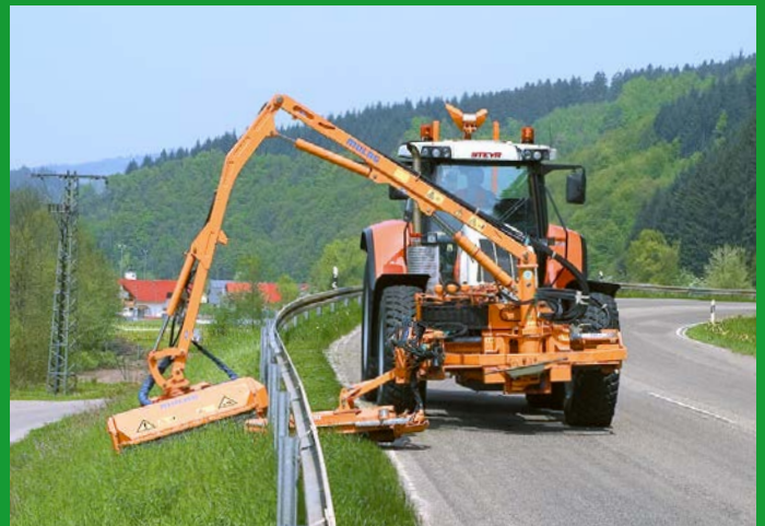
Combination mower MKM 700 in use on a crash-barrier
