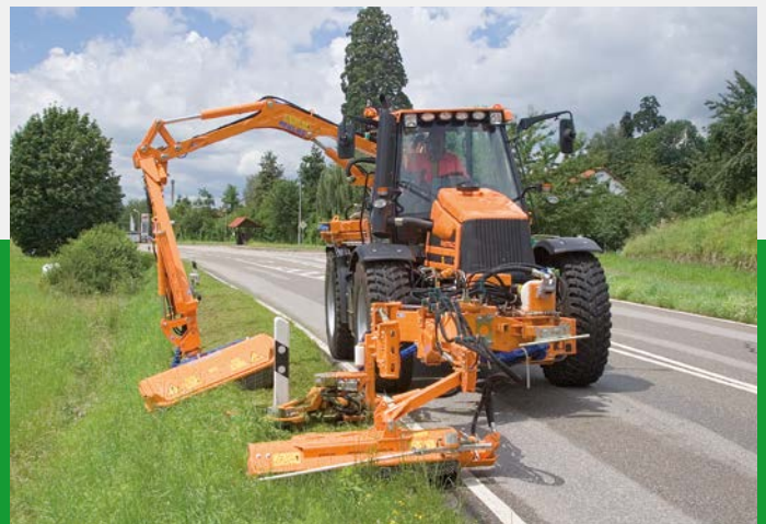
Rear-mounted mower being used in combination with a verge mower
