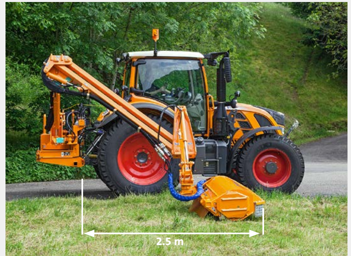
Parallelogram arm with a large swivelling range of up to 2.5 m
