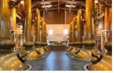
The next stop is the still house. Here, the fermented wash is filled into wash stills, where an oily liquid called low wines is produced. "We have a completely balanced distillation, which basically means one washback will fill four wash stills, which in turn will fill four spirit stills - so we don't get dummy runs or inconsistent strength of
