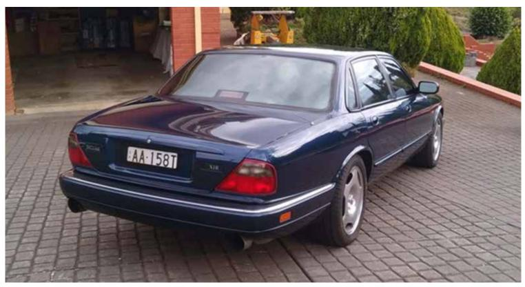
The rear of the XJR can be identified by the body-coloured boot-lid plinth, larger exhaust outlets, rear boot badge and special five-spoke "Sport" alloy wheels. The X300 XJR model is sometimes referred to as the "XJR6" to differentiate it from the later V8-engined X308 XJR.
