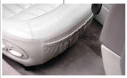
Early X300 cars were built without a front passenger glove-box and pockets on the front of the seats, due to space constraints caused by the introduction of a front-passenger airbag.
