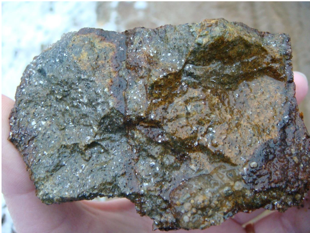
Picture of Graphitic Quartzite with about 50-70% flake graphite per volume.
