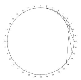
2. A 'Nephroid' is obtained in a similar fashion to that above, but this time, each point is joined to its triple (i.e. point 1 is joined to point 3, 2 to 6, 3 to 9 etc). If a value greater than 36 is obtained after tripling, 36 is subtracted as many times as necessary to get a value on the circle.
