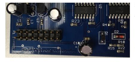
Sometimes it helps to solder just a single pin of this header, then, while heating that solder joint, move the header so that it is flat against the circuit board. Then you can go ahead and solder the remaining pins.
