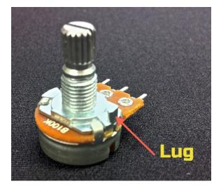
The included potentiometers feature an anti-rotation lug. You'll need to remove the anti-rotation lug. This is easy to do with a small pair of pliers. Just hold the potentiometer firmly in one hand, grasp the anti-rotation lug firmly with the pliers, and wiggle the pliers back and forth. The tab will usually break very cleanly.
