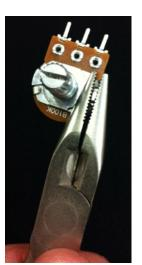
When soldering the pots to the PCB, make sure to leave just a tiny gap between the shoulders of the potentiometer pins and the PCB. If you jam the pot down tight against the PCB, over time the shoulders of the pins might wear thru the soldermask and short against the PCB traces. You can use as thin sheet of paper to space the pots up off the PCB if you like. Just remove the paper after you're done soldering!
