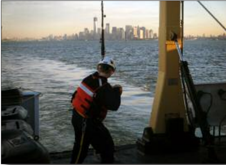
Ensign Lindsey Norman retrieves the side scan sonar that NOAA Ship Thomas Jefferson used to survey the Hudson River, so fuel barge traffic could resume. (NOAA photo)
