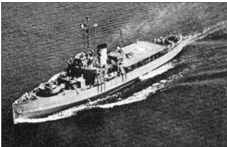
Aerial photograph of the Coast Guard cutter Cobb during World War II. Cobb served as the first test platform for landing helicopters on board ships. (U.S. Coast Guard Collection)
