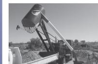
A "Blower" is constructed from an old truck which produces a vacuum strong enough to suck large rocks. The quickest and most effective way of dirt removal.
