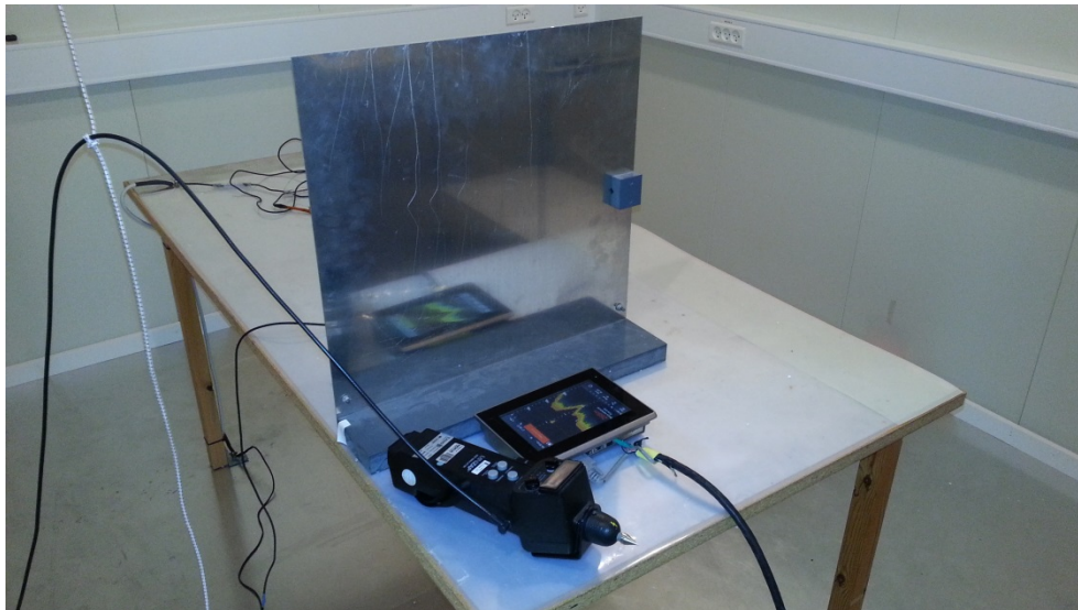
Photo 36. ESD test setup.
