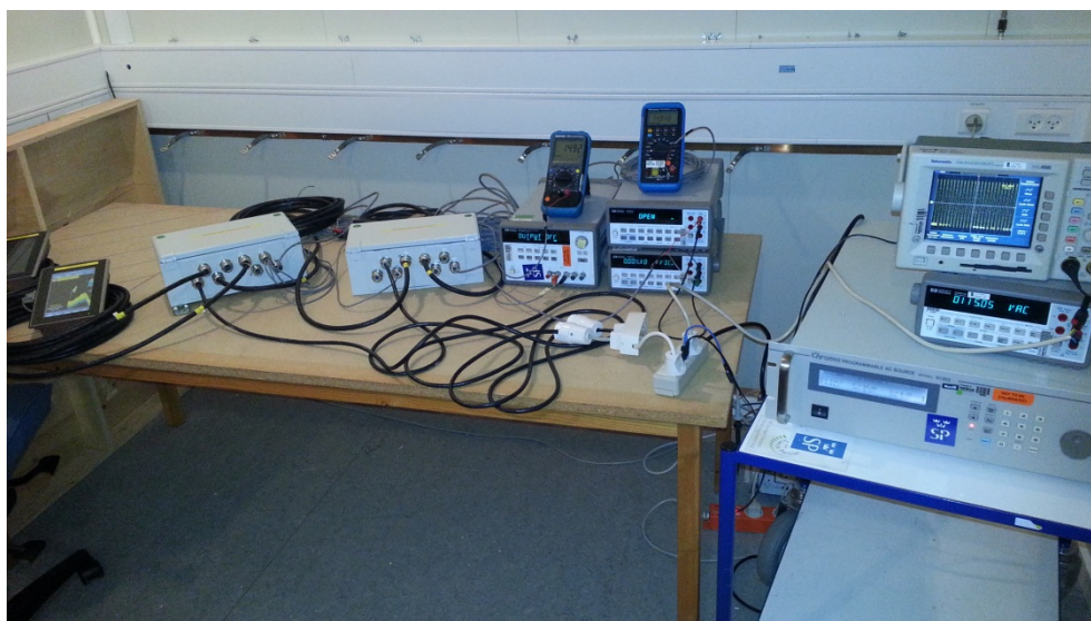
Figure 18. Power supply variations (transient) test setup.
