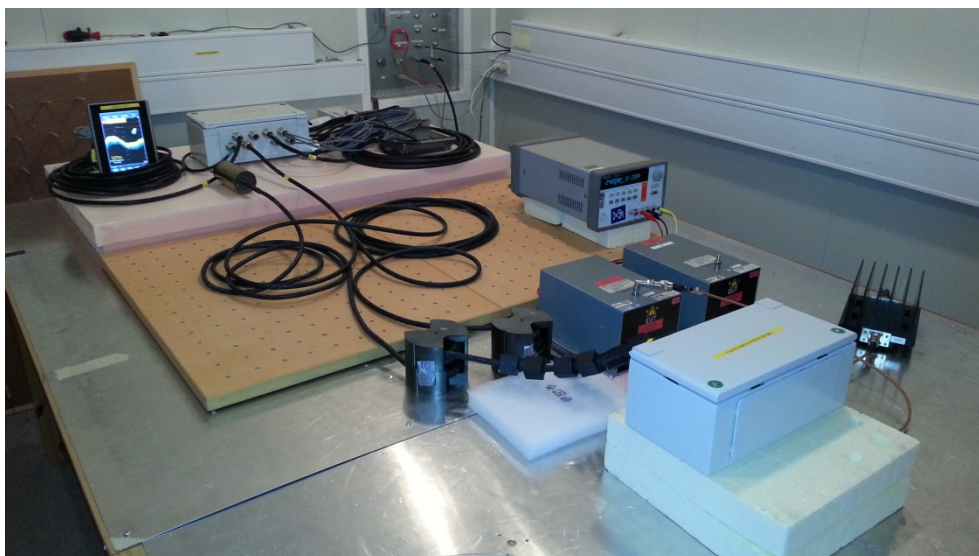
Photo 29. Conducted radio frequency interference test setup. DC power.
