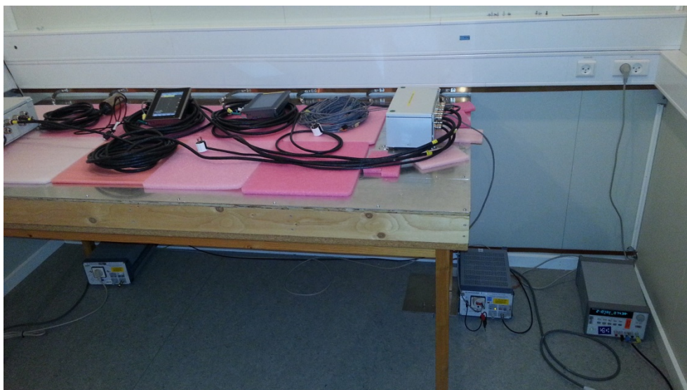
Photo 15. Conducted emission test setup. DC voltage.
