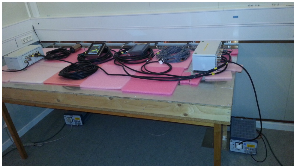
Photo 14. Conducted emission test setup. AC voltage.
