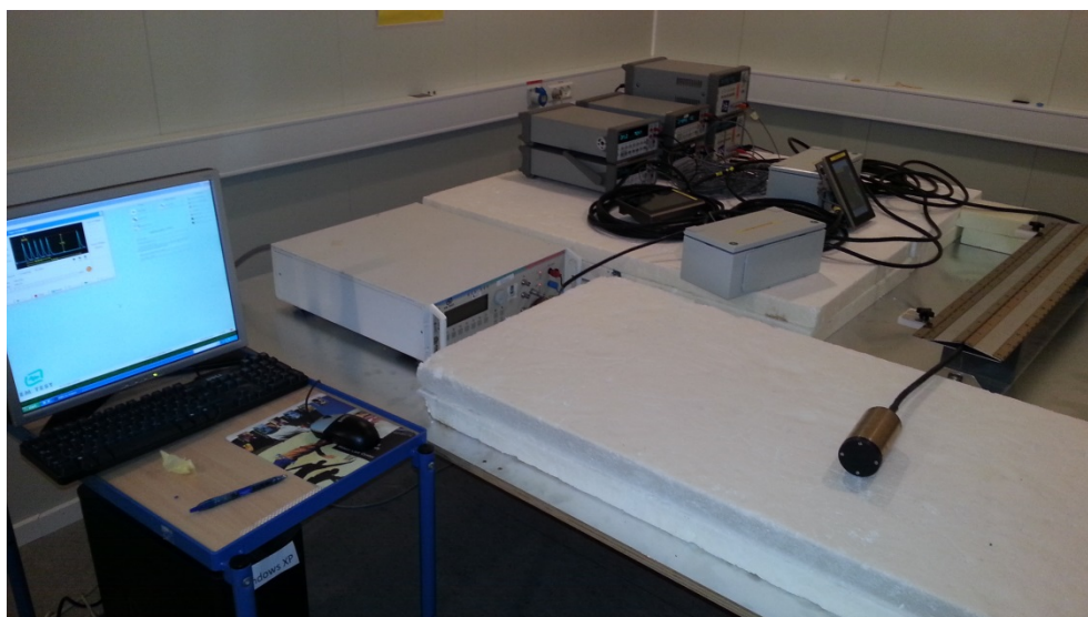
Photo 35. Burst / Fast transients test setup.
