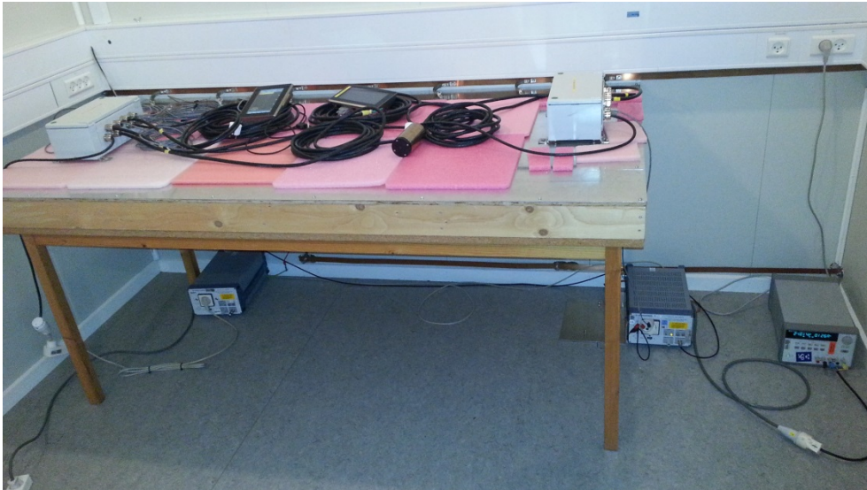
Photo 18. Conducted emission test setup. DC voltage.
