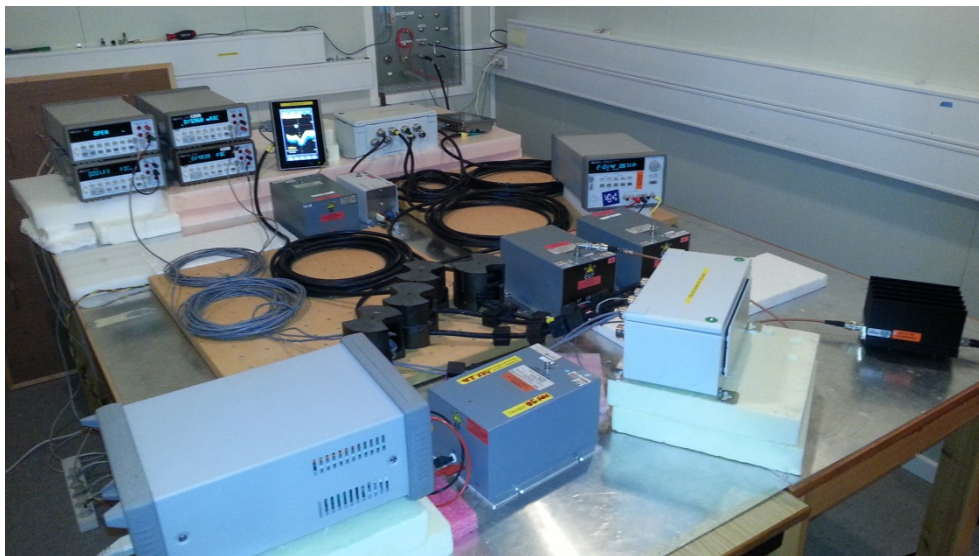
Photo 26. Conducted radio frequency interference test setup. DC power.
