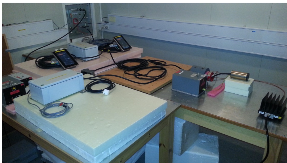
Photo 31. Conducted radio frequency interference test setup. Clamp injection on signal cable.
