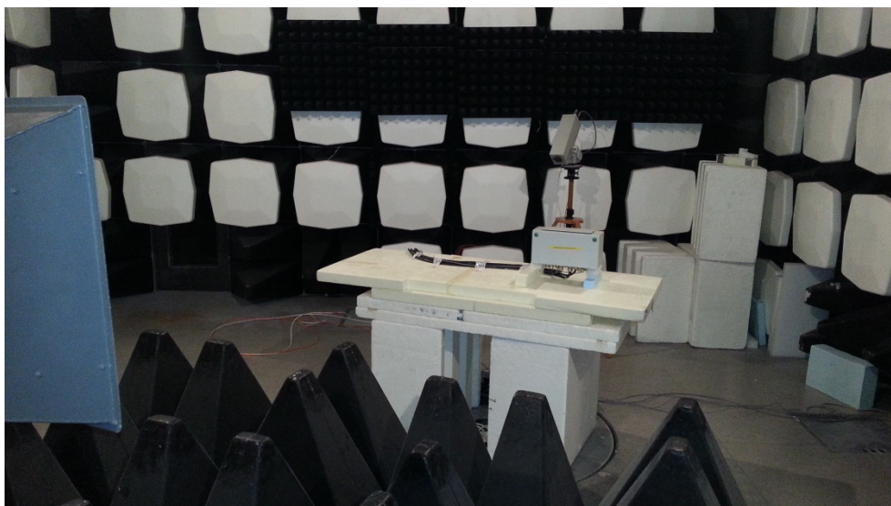
Photo 23. Radio frequency electromagnetic interference. 1 GHz – 2 GHz.
