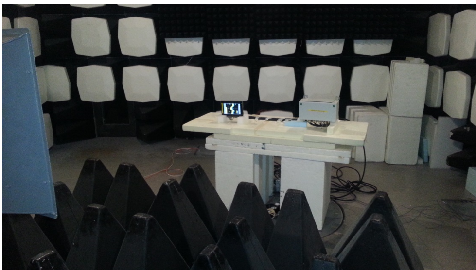
Photo 21. Radio frequency electromagnetic interference. 1 GHz – 2 GHz.
