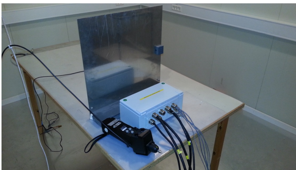
Photo 38. ESD test setup.
