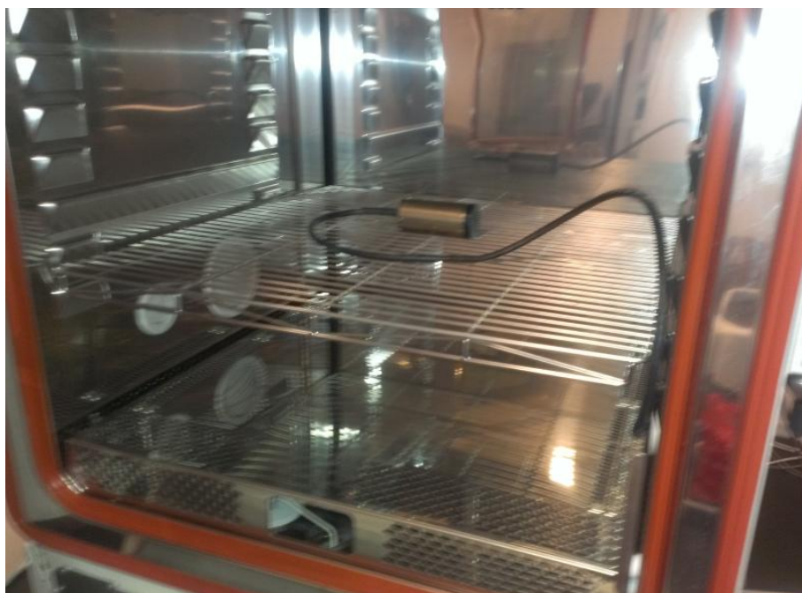
Photo 47. Test setup for Dry Heat, Storage, for Sensor Unit.
