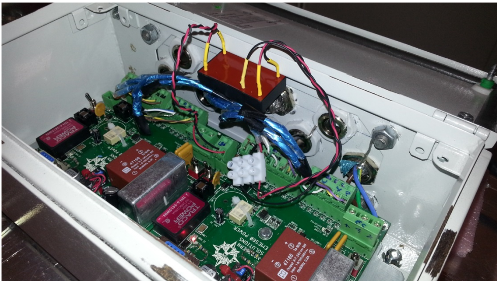
Photo 19. Shaffner filter used for DC test.
