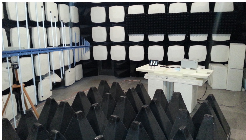
Photo 20. Radio frequency electromagnetic interference. 80 MHz – 1000 MHz.
