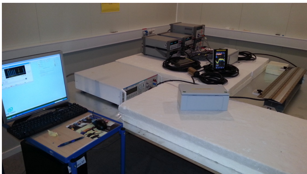
Photo 34. Burst / Fast transients test setup.
