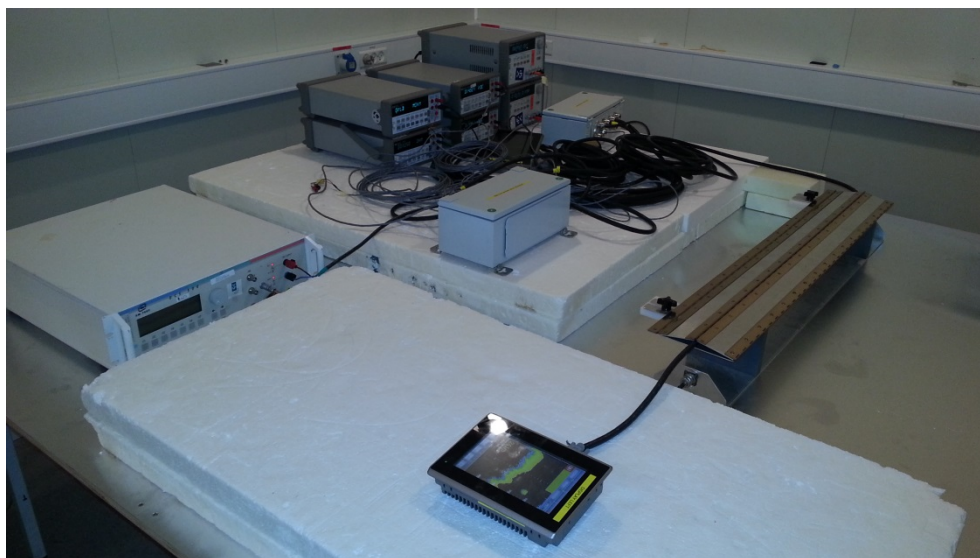
Photo 32. Burst / Fast transients test setup.
