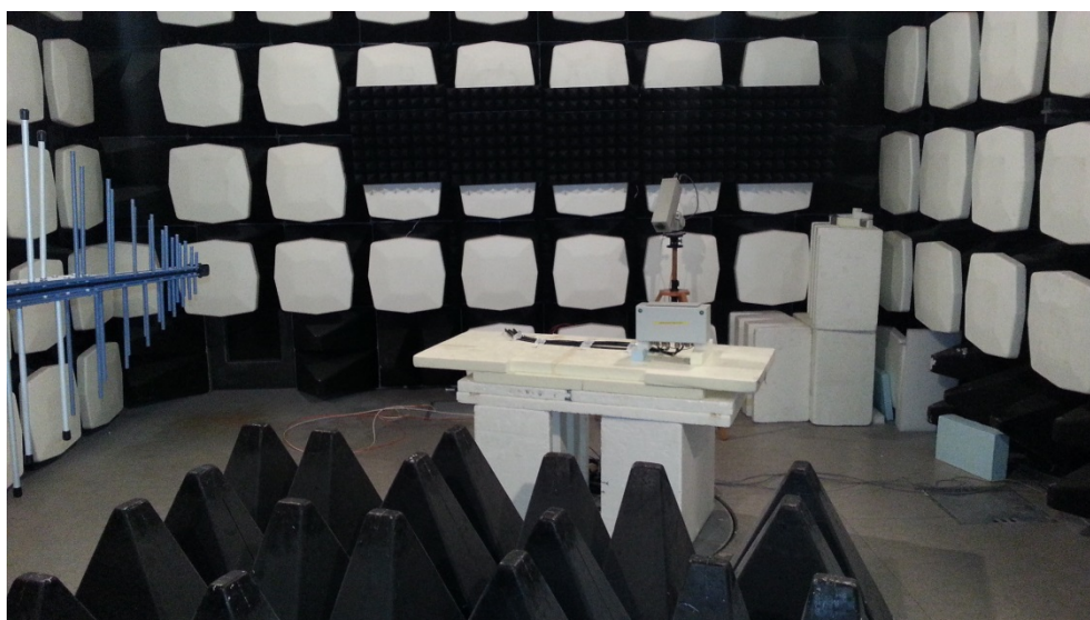
Photo 22. Radio frequency electromagnetic field 80 MHz – 1000 MHz.
