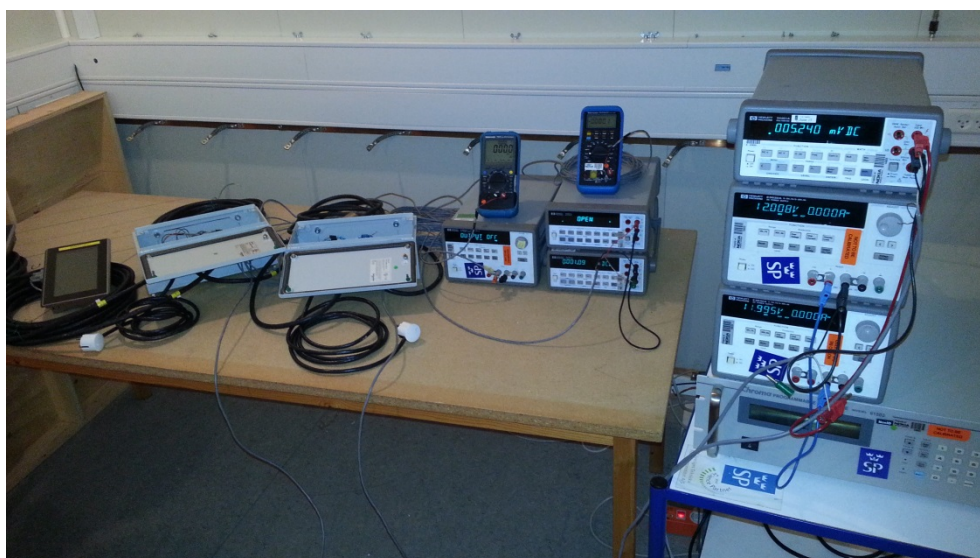
Photo 42. Test setup for power supply failure. DC power.
