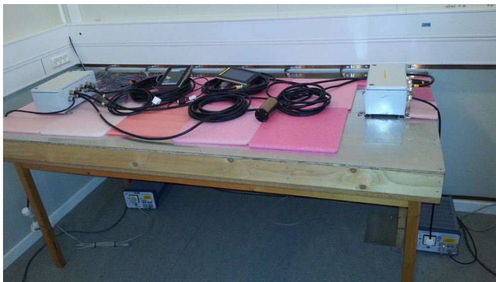
Photo 17. Conducted emission test setup. AC voltage.
