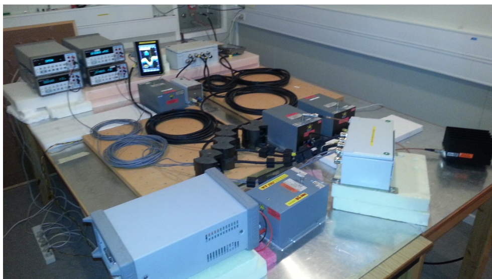
Photo 25. Conducted radio frequency interference test setup. AC power.
