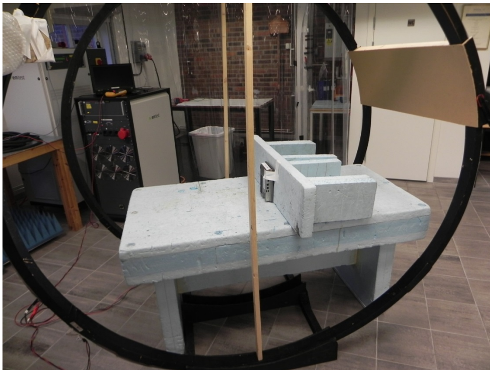
Photo 69. Magnetization in Helmholtz coil.
