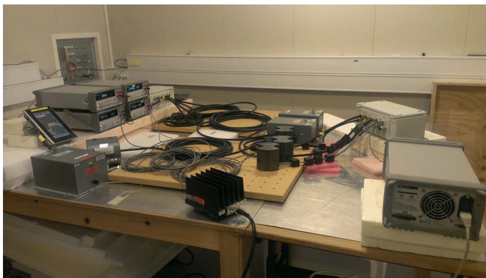
Photo 24. Conducted radio frequency interference test setup. Clamp injection on signal cable.
