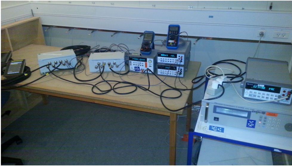
Photo 43. Test setup for power supply failure. AC power.
