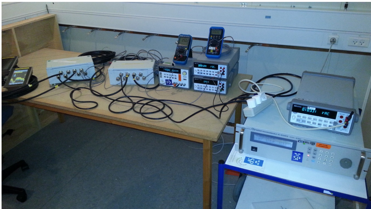
Photo 45. Test setup for extreme power supply. AC power.
