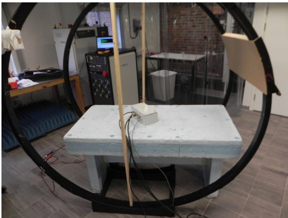
Photo 73. Magnetization in Helmholtz coil.
