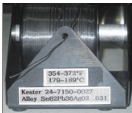
Figure 5 — Not all solder is created equal. Avoid lead-free solder — unless the kit manufacturer recommends it. Different tin-lead alloys have different melting points — make sure that you get the one that is appropriate for your kit (see text).
