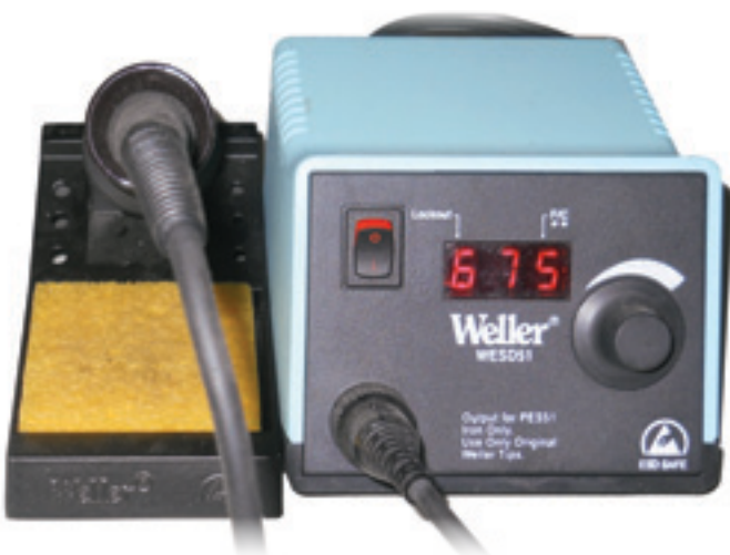
Figure 4 — A temperature controlled soldering station, such as this Weller WESD51, is highly recommended for kits that require soldering of solid state devices.
