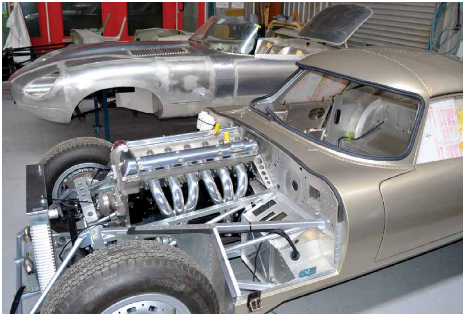
What a thrilling sight this is in the Concours Sportscar Restoration workshops near Newcastle north of Sydney. Phil Smart's new Low Drag all-aluminium bodied Lightweight E-Type with its paint applied and wide-angle 4.2 litre XK engine fitted and his Lightweight race-car in the background. Gavin King and his team garnered a huge amount of information before beginning these projects.
