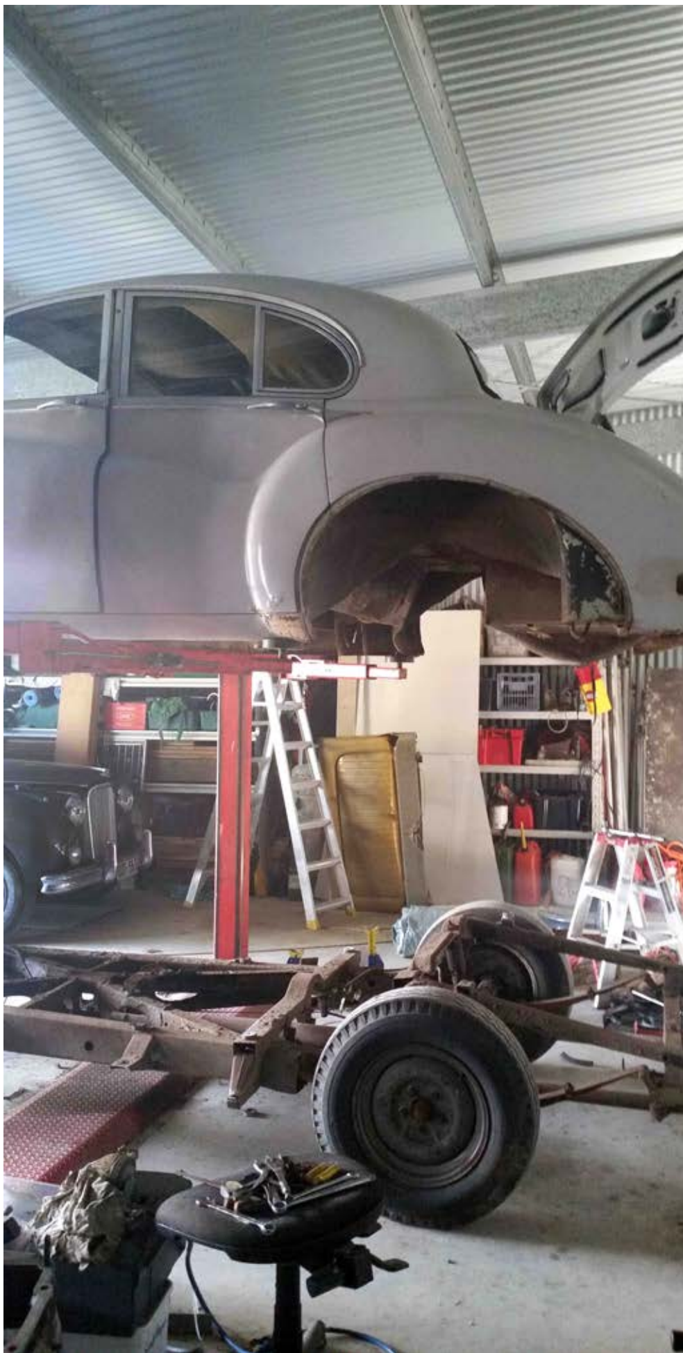
John's Mark VII M undergoing a body off restoration.
