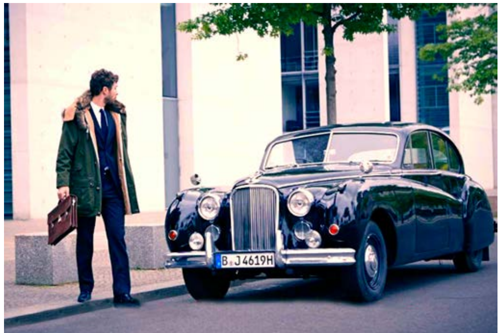
European advertisement for 1954 Mark VII M. It can be distinguished from its predecessor by the circular grilles installed below the headlights and auxiliary lamps mounted on the bumper which now wraps further around the sides of the car. Also visible are flasher type traffic indicators that replaced semaphore arms previously located between the doors.
