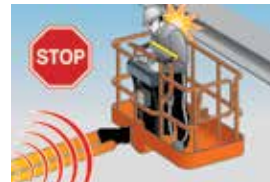
Audible alarm sounds upon operator contact with the bar.
