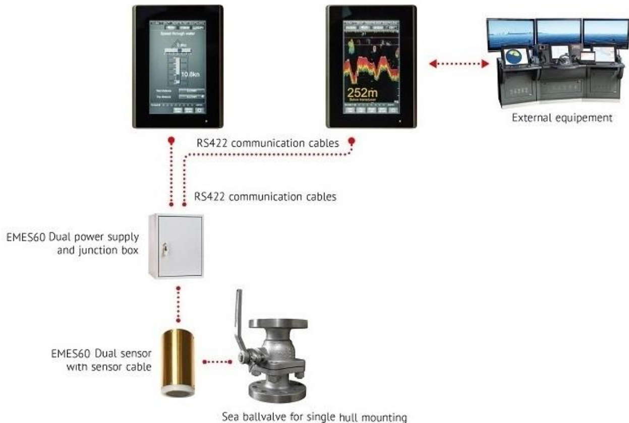
EMES60 Echosounder and Speedlog Redundant HMI units
