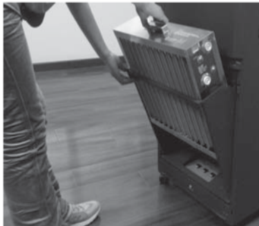
6-4 Removing the cell
