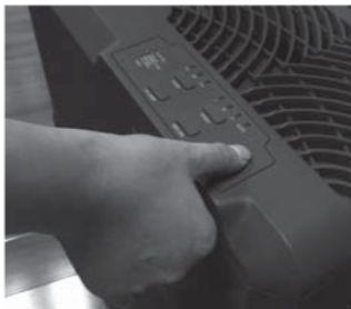
Reset the CLEAN CELL indicator light
