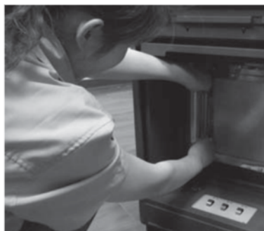
6-6 Replace the UV Lamps
