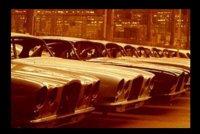
The MK X employed monocoque construction. Monocoque, translated from the French, means "single shell." The monocoque principle had been applied to aircraft design in an attempt to combine the greatest possible strength with the lightest possible weight. Jaguar had also used monocoque design in the E-Type, incorporating aerodynamic styling which was unlike anything in mass production at the time. Monocoque helped the E-type become the fastest production car that you could buy in 1961.
