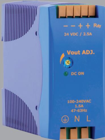
The PSU 6R is the ideal choice for your control supply needs for the DFE (above 97A) Soft Starters. It is a compact 24VDC power supply that is DIN Rail mounted which cuts down on cabinet space and minimises installation time.
