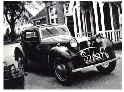
Rare photo of a 1932 SSII (Series 1) coupe fitted with a curved headlight bar. This series was the last SS/Jaguar model to have a 3-speed manual gearbox. As with many pre-war cars, the survival rate was very low.
