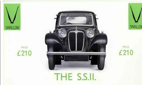
**BUMPERS.** Exceptionally substantial and of attractive appearance are domed  $2\frac{1}{2}$  in section. Those at the rear are of the quarter type. **COACHWORK.** Coachbuilt, with leather grained head and large travelling trunk, the body represents the finest example of craftsmanship.
