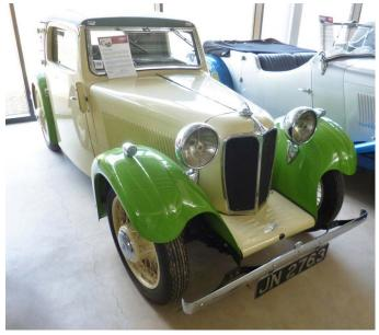
1933 SSII (Series 2) coupe with the headlights fixed to the mudguards. 1934 SSII's were fitted with sweeping wings. No SSII's are believed to have been imported (or exist) in Australia.
