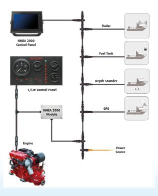
Beta Marine & Actisense have developed an interconnection module to facilitate an interface that will connect a Beta Marine C or CW engine control panel with an NMEA 2000 network. This module simply "T" connects between an engine and engine control panel & converts information to a NMEA 2000 network friendly format.
