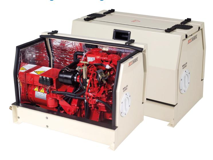
Beta Marine has gained considerable experience over many years of manufacturing marine generating sets for yachts and work boats. These small marine generating sets are based on Kubota diesel engines with marine rated "generators" offering 4 kVA up to 58 kVA; and available as a standard open generating set or acoustically housed.
