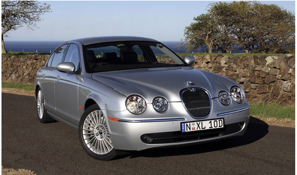
The 2006 X206 S-Type introduced a 2.7-litre twin-turbo-diesel V6 engine. The X206 S-Type could be identified by its bonnet-mounted 'leaper' and new tail-lights.
