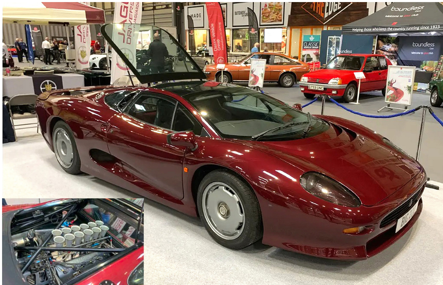
This intriguing XJ220 was displayed at the November NEC Classic Motor Show at none other than the UK Jaguar Drivers' Club stand. Having started life as prototype chassis no 005, it was modified by marque specialist Don Law in 2000, who turfed out the V6 used in the production cars in favour of the Jaguar V12 engine it had originally been designed to use, even finding a four-cam prototype V12 engine to make a proper job of it. (Also see NEC Auction results pages 52-53).
