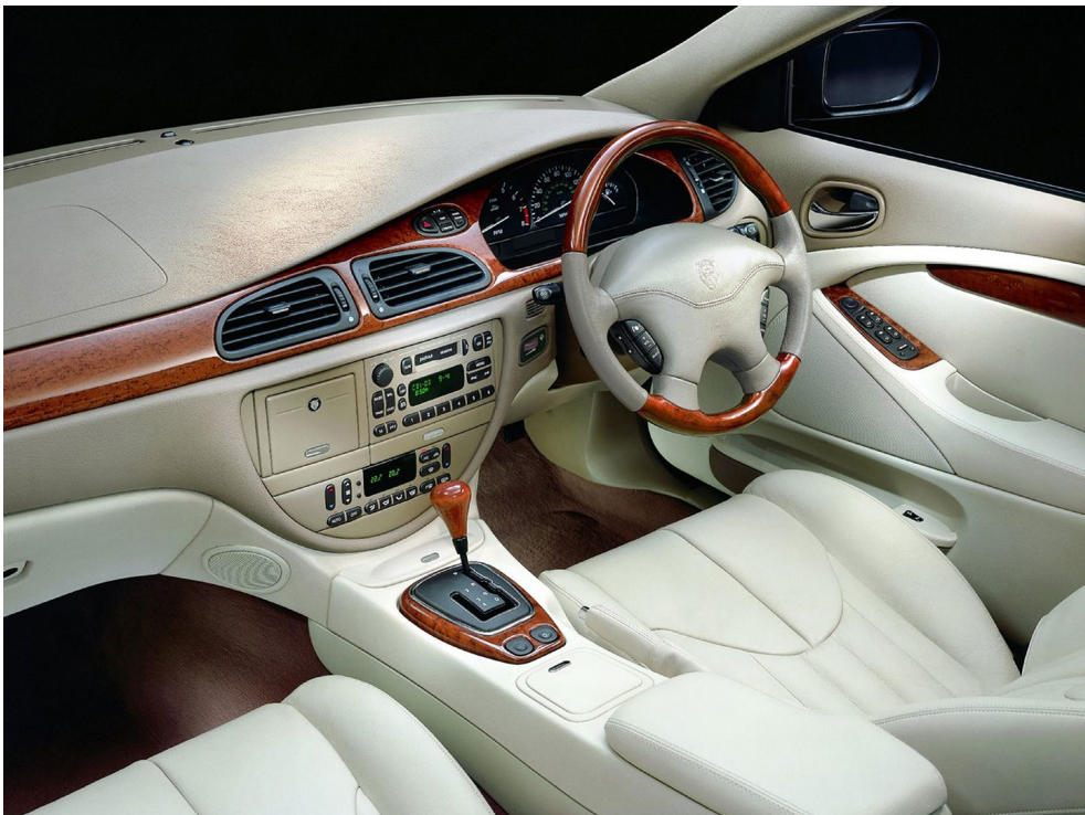
1999 X200 S-Type interior showing U-shaped centre console (replaced in the X202).
