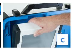
7. Seat the tablet in the cradle (A), tilt it back (B), and lock it in place (C). ▼
