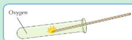
Fig. 25.10 Oxygen relights a glowing splint. This is the characteristic test for oxygen.
