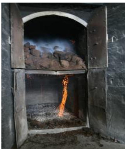
Peat burning in the kiln at Laphroaig, giving off smoke that is drawn up in to kiln floor above to “infuse” into the barley.
